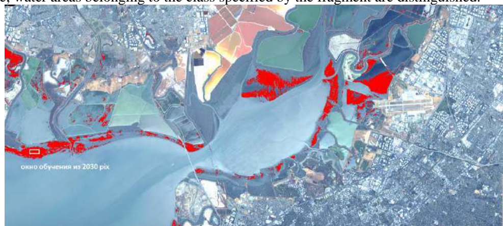
Figure 4. HSI Moffett Field with automatic classification by training window (shown with white frame on the left side of the image).
