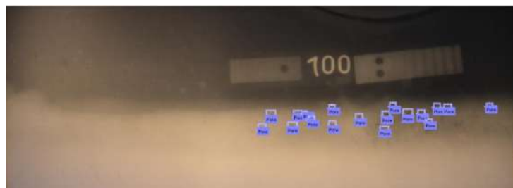
Figure 13. Selection of areas of interest in the form of defects “Pore”.
