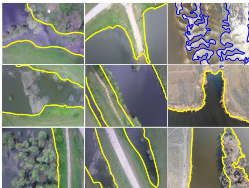
Figure 5. The vectorization of water bodies images with UAV. The colored lines show the boundaries of the reservoirs.
