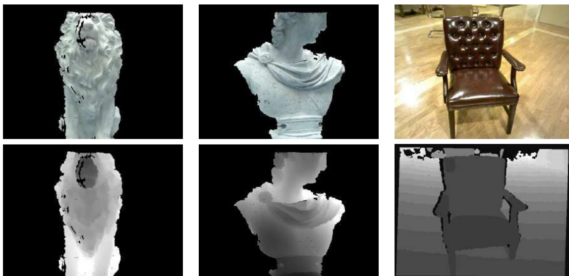
Figure 1. RGB images and depth maps of a lion, an apollo, and a chair are scanned by Kinect sensor.
