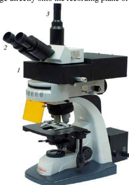
Figure 1. Microscope-based AO spectral imager. 1 – AO spectral imaging unit, 2 – eyepieces for visual observation, 3 – color camera for wideband image registration.
