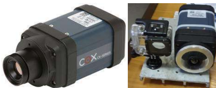
Figure 2. COX-1000 IR camera and its mounting on the same platform with GoPro box.
