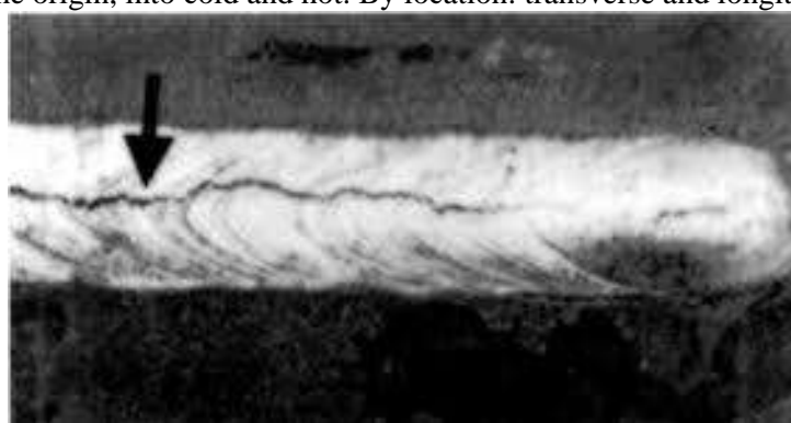
Figure 3. Crack in welded joint.
