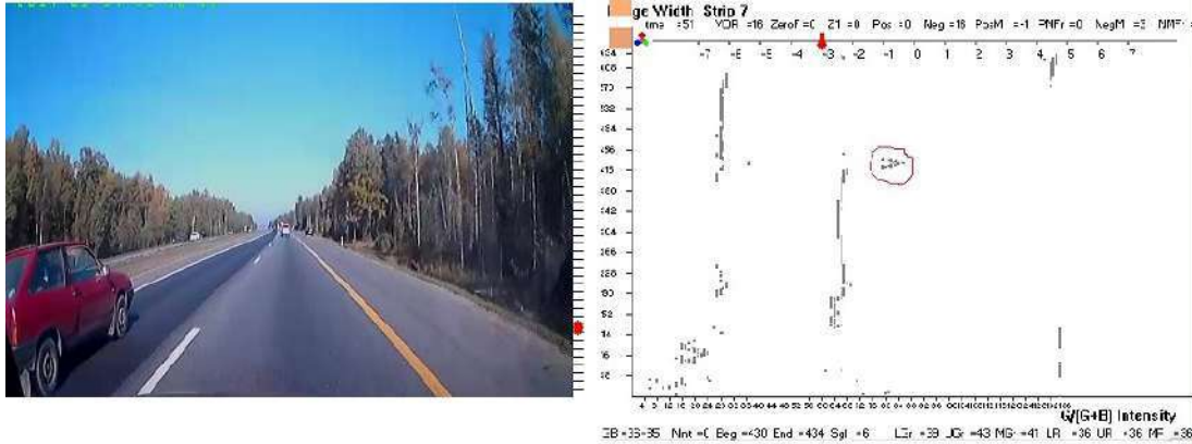
Figure 2. A road scene and the geometrized histogram of the color image of the 7-th horizontal strip.
