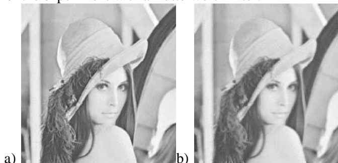
Figure 3. Filtered image of "Lena": radially symmetric SE-filter with blurs(a) \sigma = 3 , (b) \sigma = 5 .
