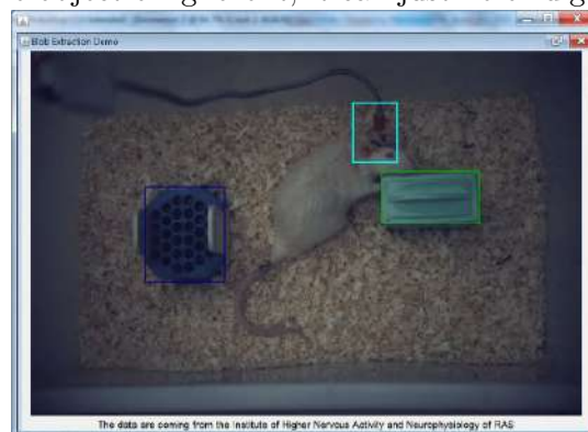
Figure 1. A laboratory rat investigates a new object in the cage. The logic program has detected three blobs in the video: EEG cap that connects the head of the rat with EEG cable; a new green object; and a new blue object placed in the cage.
