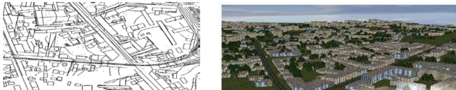
Figure 7. A fragment of the electronic map and a 3D model built on the basis of the attributive information of the digital map.
