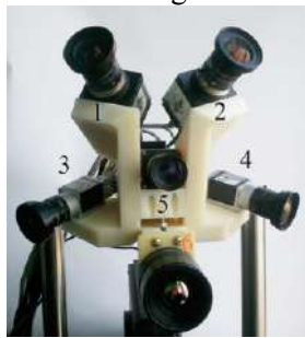
Figure 1. RPM layout cameras: LWIR (bottom center) and five TV.
