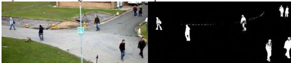
Figure 1. Detection of a moving person on a video sequence: the frame of the original video sequence (on the left), the formed mask (on the right) [10].
