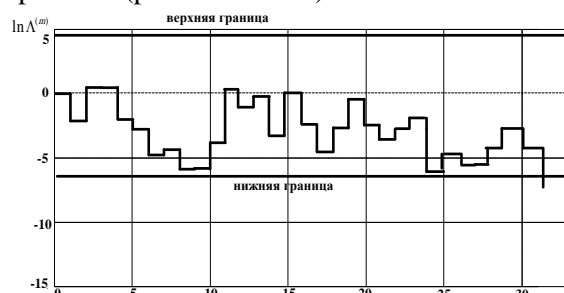
Figure 3. The values of likelihood ratio at each step of observation with respect to the decision limits (onset of inspiration registered at count 31).
