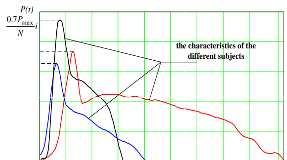
Figure 5. Examples of the different characteristics of the pressure in the breathing circuit at the relay type of impact (expiratory phase).
