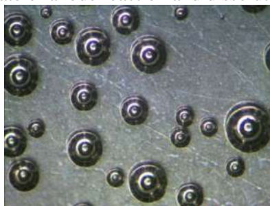
Figure 1. The snapshot of the aluminum surface at a corrosion potential in 0.1 M NaCl (pH 11).
