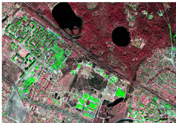
Figure A1. The result of building extraction using the trained U-Net model (image, dsm) for the image with the size of about 5 \times 5 km and 1-m resolution. Detected buildings are displayed in green.
