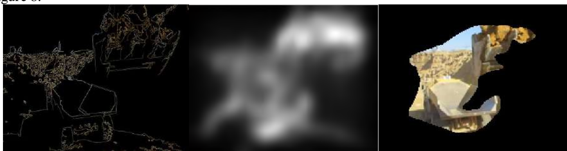
Figure 8. Left. Preprocessing an image using the Sobel operator. The middle. Map of the importance of the image. On right. The selected area of the image.
