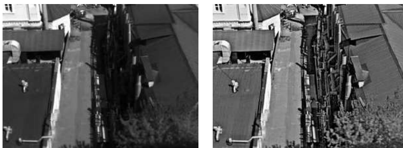
Figure 4. Multiscale Retinex results (observation conditions – sunny day): left – original frame, right – after Multiscale Retinex.
