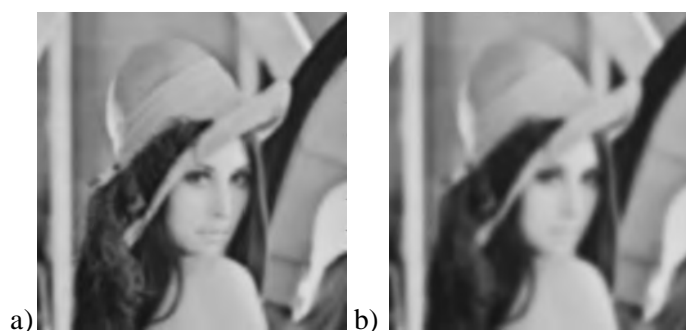
Figure 4. Filtered image of "Lena" by the Butterworth filter with blur (a) \sigma = 3 , (b) \sigma = 5 .
