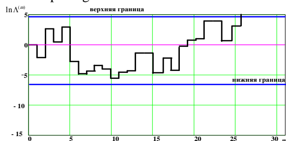
Figure 2. The values of likelihood ratio at each step of observation with respect to the decision limits (onset of inspiration registered at count 26).
