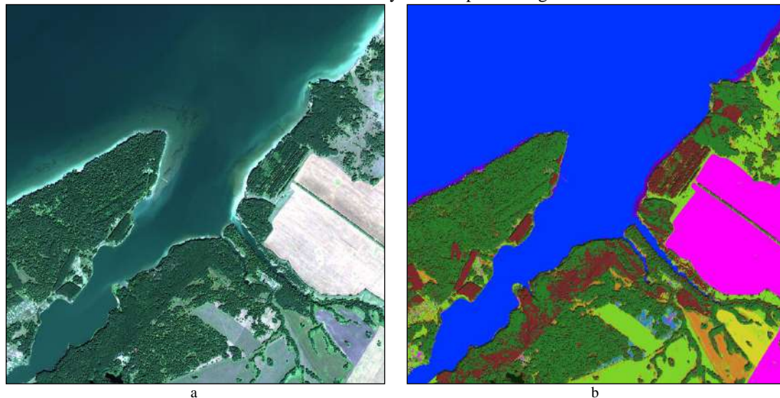
Fig. 5. RGB-composite (bands 5, 3, 2) of the WorldView-2 satellite image (a) and segmentation result obtained by ECCA clustering algorithm (b).
