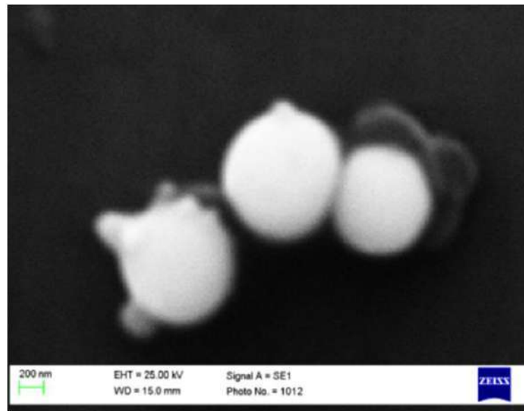
Fig.2. SEM image of gallium particles obtained by laser ablation in ethyl alcohol.
