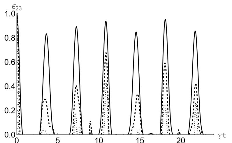
**Figure:** 3) The entanglement  $\varepsilon_{23}(t)$  as a function of a dimensionless time  $\gamma t$  for biseparable state (6) for  $\alpha = \frac{\pi}{4}$ . The intensity of the cavity field for graph is  $\langle m \rangle = 0.1$  (solid),  $\langle m \rangle = 1$  (dashed) and  $\langle m \rangle = 3$  (dotted).
