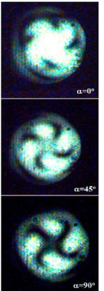
Fig.8 Experimentally obtained spiral beams under different directions of polarizer axes
