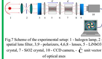
Fig.7 Scheme of the experimental setup: 1 - halogen lamp, 2 - spatial lens filter, 3,9 - polarizers, 4,6,8 - lenses, 5 - LiNbO3 crystal, 7 - SiO2 crystal, 10 - CCD camera, -  $\hat{C}$  unit vector of optical axes
