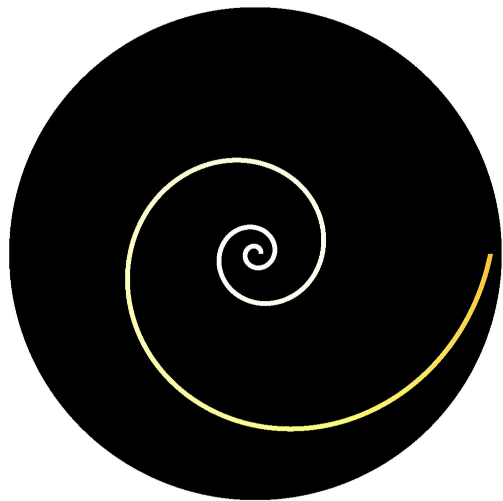
Fig. 2. Cross section of the slit in the form of a logarithmic spiral ( a = 0,022 , b = 0,2 , d = 0,1 mm, \varphi \in [0, 6\pi] )
